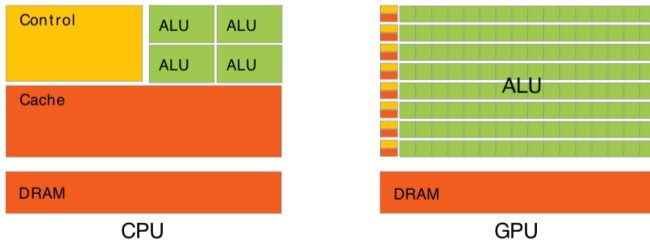
Fig. 1. Comparison of CPU and GPU [1]
